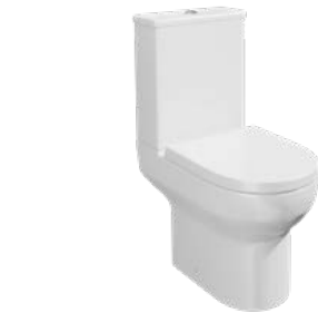
SPA RIMLESS OPEN BACK PAN INCLUDING CISTERN & D SHAPE SOFT CLOSE SEAT 360w x 815h x 625d Roughing-In 120mm | Side Clearance 100mm
